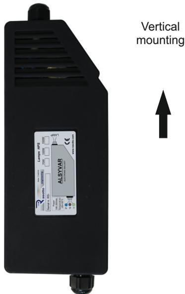
ALSYVAR is a dimmable electronic ballast designed to be housed inside the pole, away from heat sources, on street lamps, instead of the traditional ferromagnetic system. It works with high pressure sodium lamps, obtaining savings of over 60% compared to the traditional system during the nighttime operating range.
